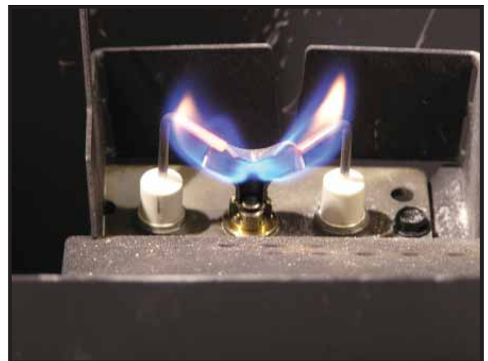
Figure 3.1 IPI Pilot Flame Patterns
