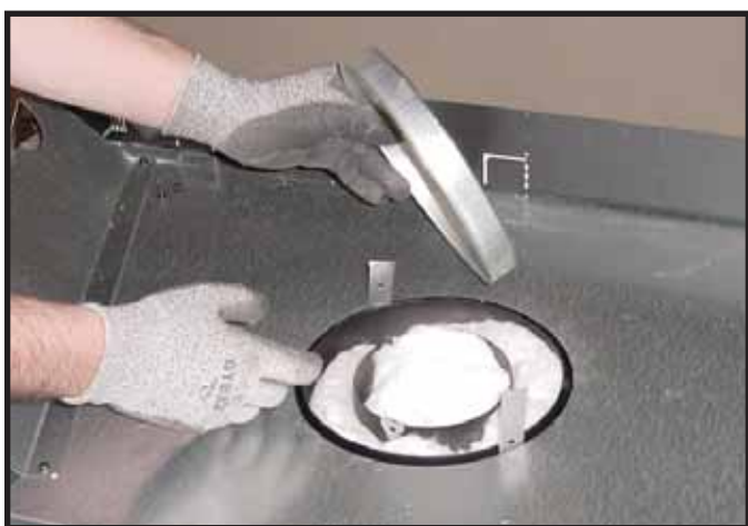
Figure 9.3 Remove the seal cap.
