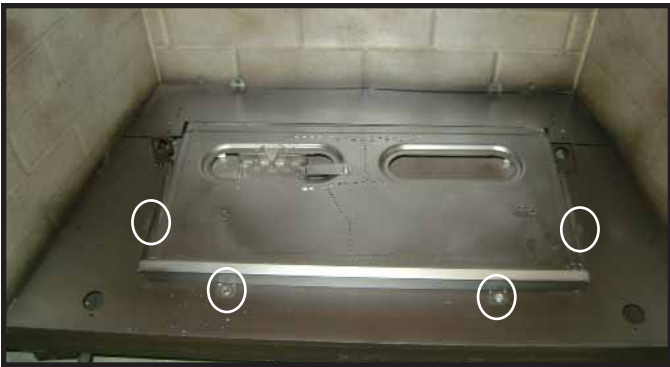
Figure 3.9 Remove Burner Skirt
