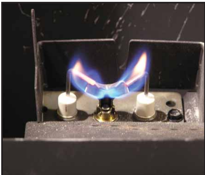
Figure 3.1 IPI Pilot Flame Patterns
