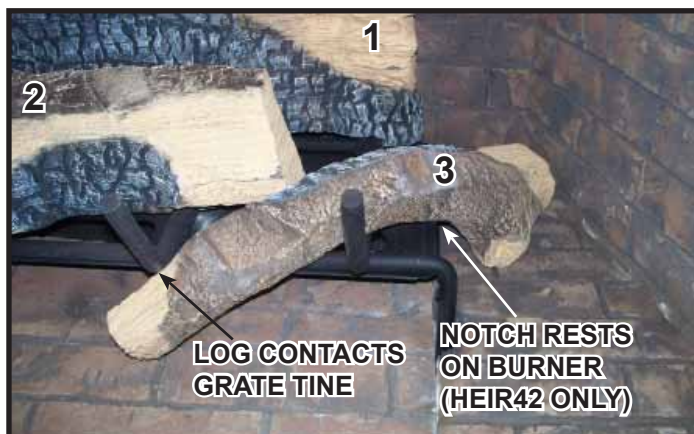
Figure 7. Log #3 Placement
