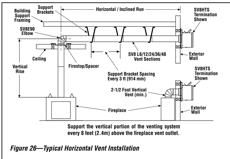
**Figure 26—Typical Horizontal Vent Installation**
