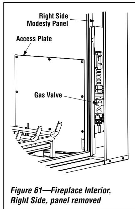
**Figure 61—Fireplace Interior, Right Side, panel removed**
