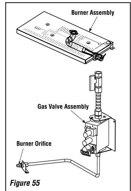
**Step 5.** Remove the control compartment access door and gasket by removing the twelve (12) screws securing it, and set it aside for later reinstallation. The gas valve can be accessed through the opening, or the complete assembly can be removed by sliding the assembly to the right.
