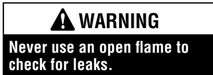
Turn on gas supply and test for gas leaks using a gas leak test solution (also referred to as bubble leak solution).
