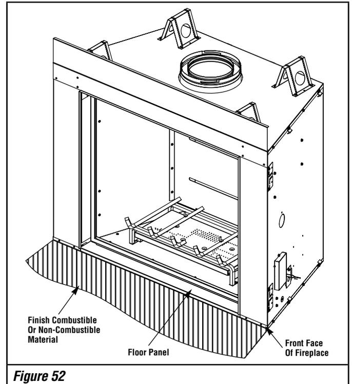
**NOTE:** A finish trim piece is shipped with your fireplace to extend the base 1/2" to be flush with the finish flanges on the side of the fireplace. This filler is shipped on top of the fireplace wrapped in foam. If desired this piece can be placed on the base of the fireplace. It is secured with bend tabs on either side. Lay the extension in front of the base then secure by bending tabs on each side over to secure to the base. While this piece is provided it is not required.
