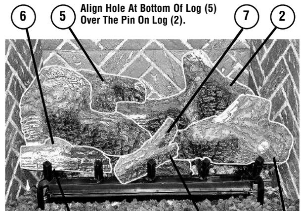
Engage Log (6) With The Grate Pin And Align Groove At The Bottom Of The Log Over The Grate.
