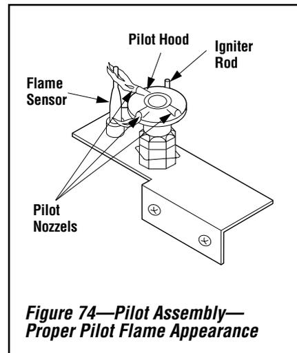
**Figure 74—Pilot Assembly—Proper Pilot Flame Appearance**
