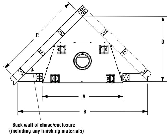
Figure 12—Corner Framing with Square Termination (SV8HTS)
