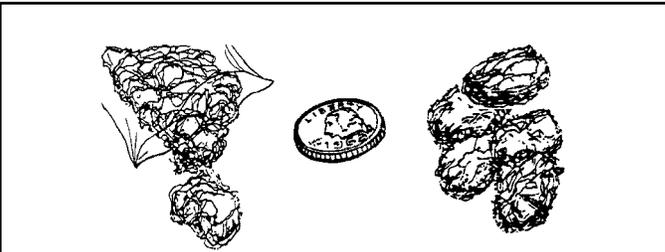
**Figure 64—Glowing Ember Separation**
