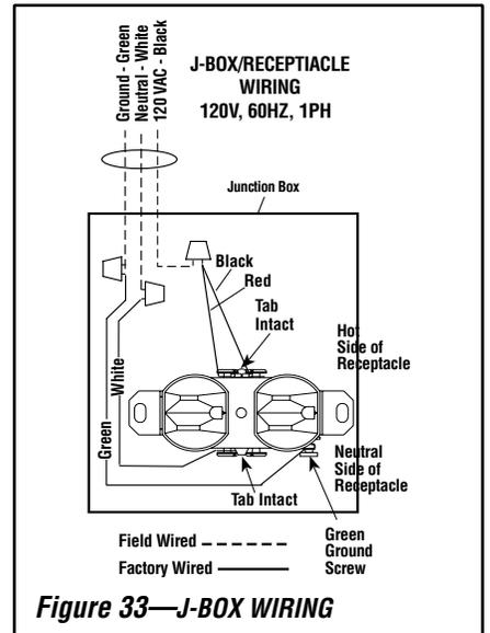
Figure 33—J-BOX WIRING
