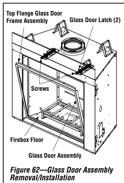
**Figure 62—Glass Door Assembly Removal/Installation**
