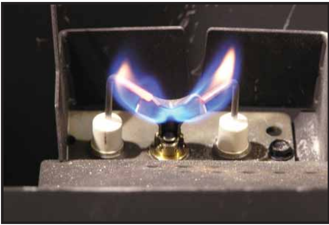
Figure 3.1 IPI Pilot Flame Patterns
