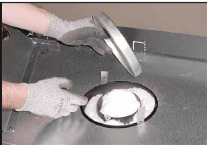
Figure 9.3 Remove the seal cap.
