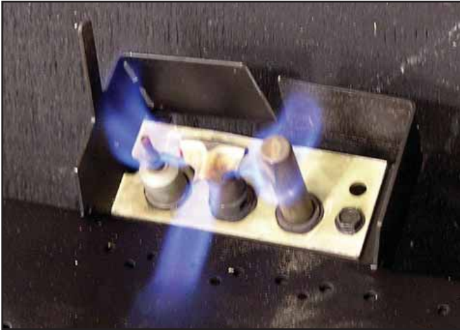
Figure 3.2 Standing Pilot Flame Patterns
