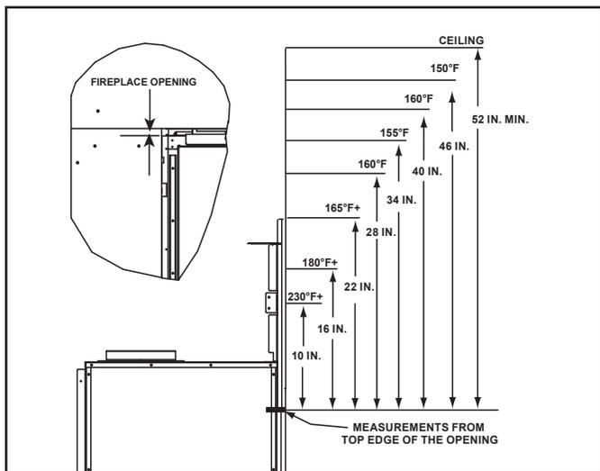
Figure 3.4 Wall Surface Temperatures
