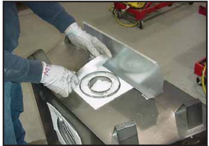
Figure 9.4 Remove the seal cap.
